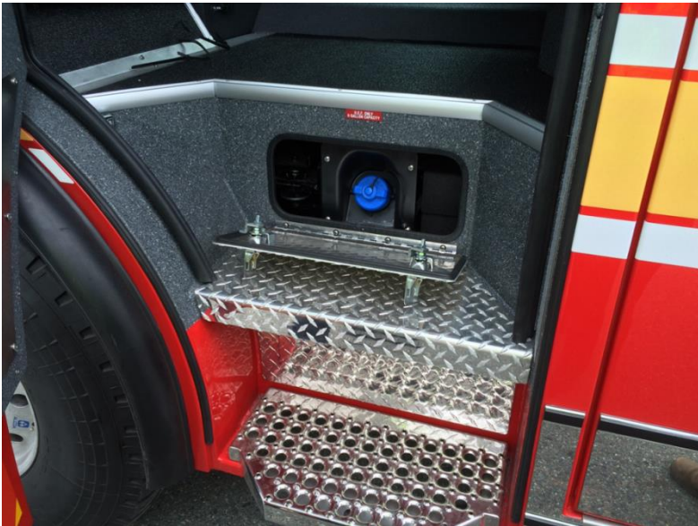
DEF fill located inside driver's side rear cab door
