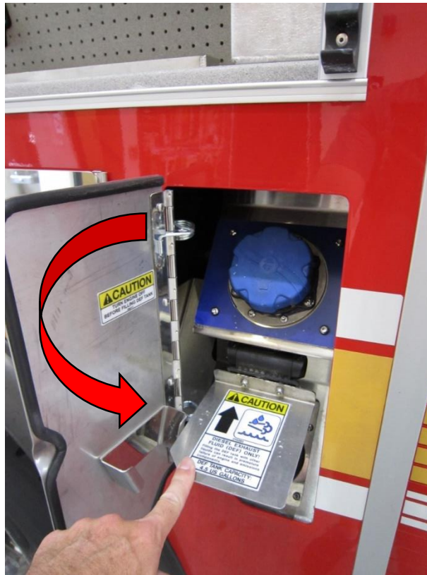
DEF fill co-located with driver's side diesel fill
